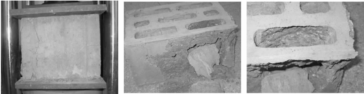
图 4 再生混凝土砌块不同部位典型的破坏面 Fig. 4 The typical breaking face of recycled concrete hollow blocks
