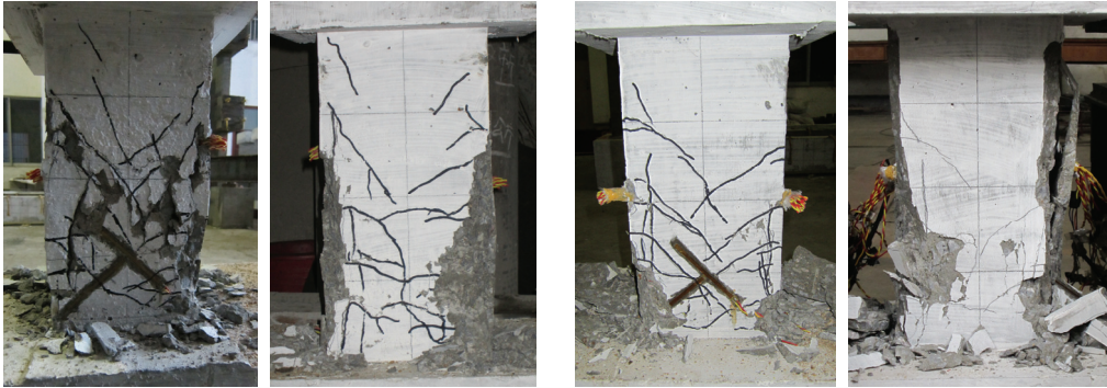
图 1 剪切黏结破坏 Fig.1 Shear bond failure
