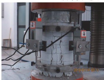
Fig.2 The equipment set-up for the loading test
