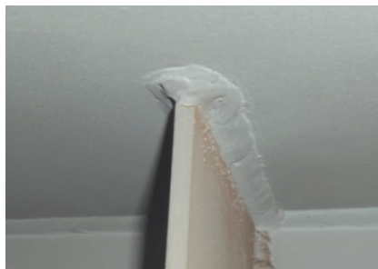
图1 竖向加劲肋与顶板焊缝 Fig.1 Vertical stiffener and plate weld
