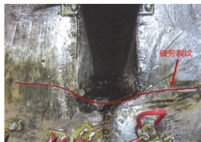
图2 疲劳裂纹开展路径 Fig.2 Fatigue crack growing path
