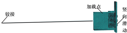
图 4 腹板双角钢连接梁柱子结构数值模型 Fig.4 Numerical model of beam-column substructure with double web angles connection
