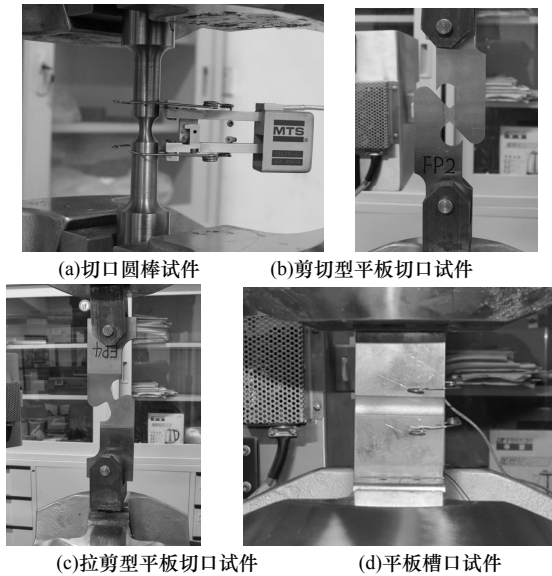
图6 试验中各切口试件加载图 Fig.6 Loading on the tested specimens
