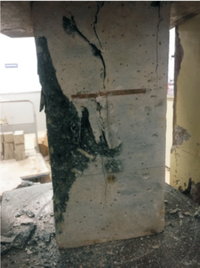
图 5 混凝土轴心抗压破坏情况 Fig. 5 Failure mode of SCASC after uniaxial compressive strength test
