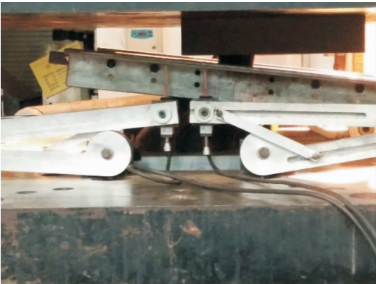
图 6 试验照片(2号支座, 组合 3, 罩橡胶套) Fig. 6 Test photo (No. 2 bearing, combination 3, cover with rubber bush)
