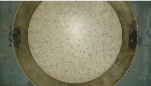
图 7 中空连接钢板损伤(Q345B) Fig. 7 Damage of the hollow connecting steel plate(Q345B)
