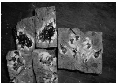
图 2 钢纤维混凝土经微波照射 6 min 冷却后截面图 Fig.2 A cross-sectional view of steel fiber reinforced concrete by microwave irradiation after 6 min cooling
