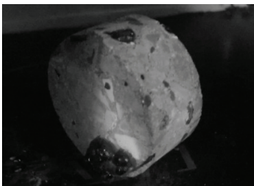
图 1 钢纤维混凝土经微波照射 6 min 时状态图 Fig.1 Steel fiber reinforced concrete under microwave irradiation at 6 min state
