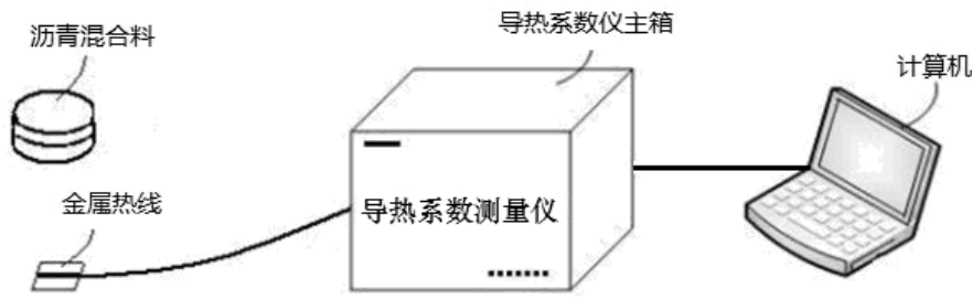
图 1 导热系数瞬态热线法测试装置示意图 Fig.1 Testing system of transient hot line thermal conductivity coefficient
