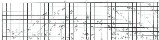
图 6(f) HJJL-3 裂缝开展图 Fig 6(f) Crack development figure of HJJL-3
