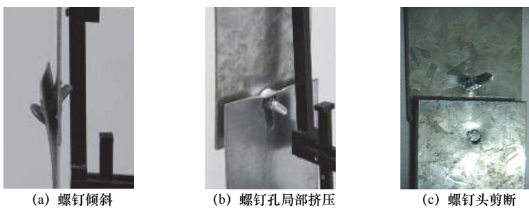
图 4 钢板与钢板连接的破坏特征 Fig.4 Failure modes of connection between steel and steel
