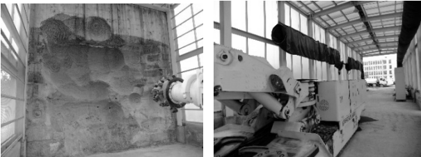
图1 人工岩壁试验场及试验掘进机 Fig. 1 Artificial rock test field and experimental road header
