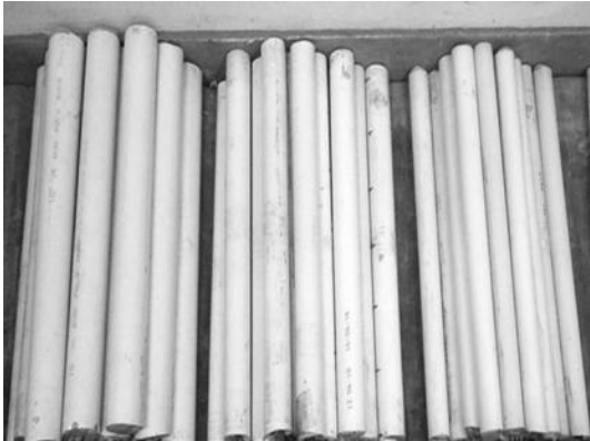
图 4 三种直径的微型桩 Fig.4 Micropiles of three different pile diameters
