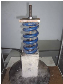
图2 持载的粘结试件 Fig.2 Bond specimen with sustained load 表3 钢筋持载值(kN) Tab.3 The sustained load value of steel (kN)
