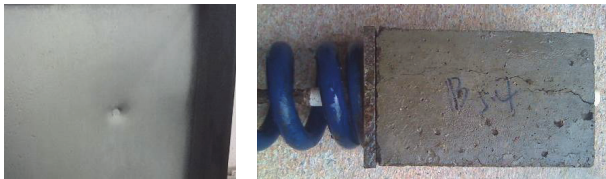
图4 持载50%粘结试件冻融过程破坏 Fig.4 Frost damage of specimens at 50% load level
