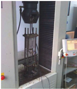
图3 拔出试验加载装置 Fig.3 Loading set-up of pull-out test
