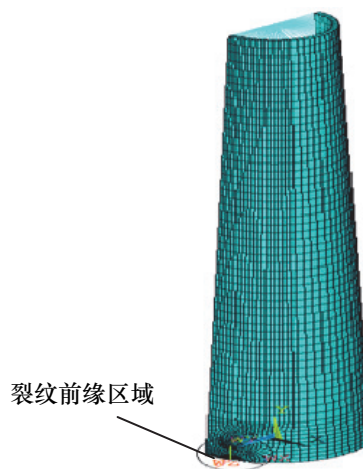
图3 梭形变截面薄壁圆柱壳有限元计算模型 Fig.3 The finite element calculation model of thin walled shuttle cylinder structure
