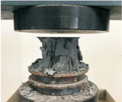
图 4 D46-PE0 试块破坏模式—脆性劈裂 Fig. 4 Failure mode of D46-PE0—splitting failure
