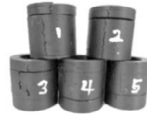
图 4 FFF-CFRP 锚环破坏形态 Fig. 4 FFF-CFRP anchor ring damage pattern
