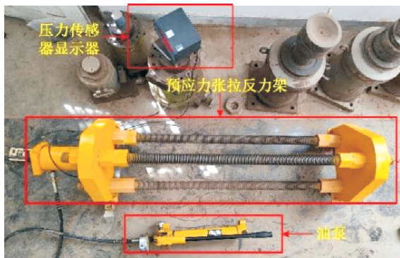
图 3 FFF-CFRP 锚环张拉锚固破坏试验装置 Fig. 3 FFF-CFRP anchor ring tension anchoring failure test instrument
