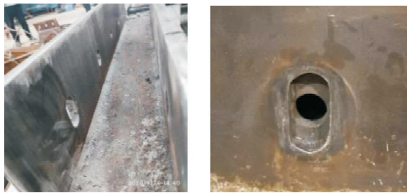
图 9 装置部件磨损情况 Fig. 9 Wear condition of device components
