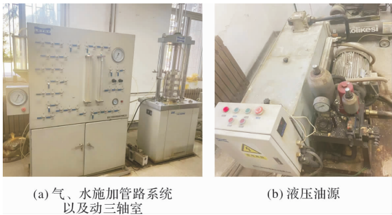
图 1 TYS-20 型微机控制电液伺服土动三轴试验机 Fig. 1 TYS-20 microprocessor controlled electrohydraulic servo soil dynamic triaxial testing machine
